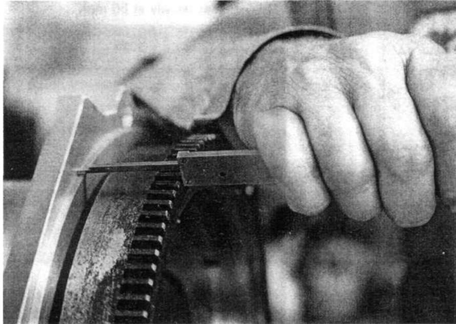
The second number is a measurement of torque. The hub is attached to the flywheel using the original bolts. These are special hardened bolts. When installing them, use a torque wrench and the torque numbers in the manufacturer's service manual.
