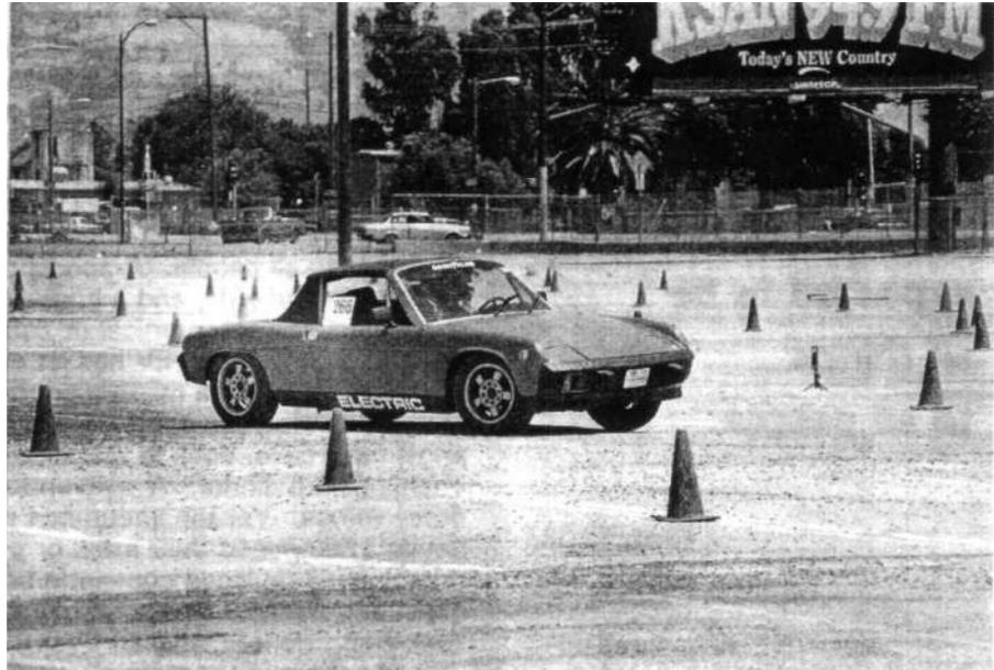
This high-performance electric sports car (a converted 914 Porsche) has a top speed of 90 mph and a range of over 120 miles on a single charge.
