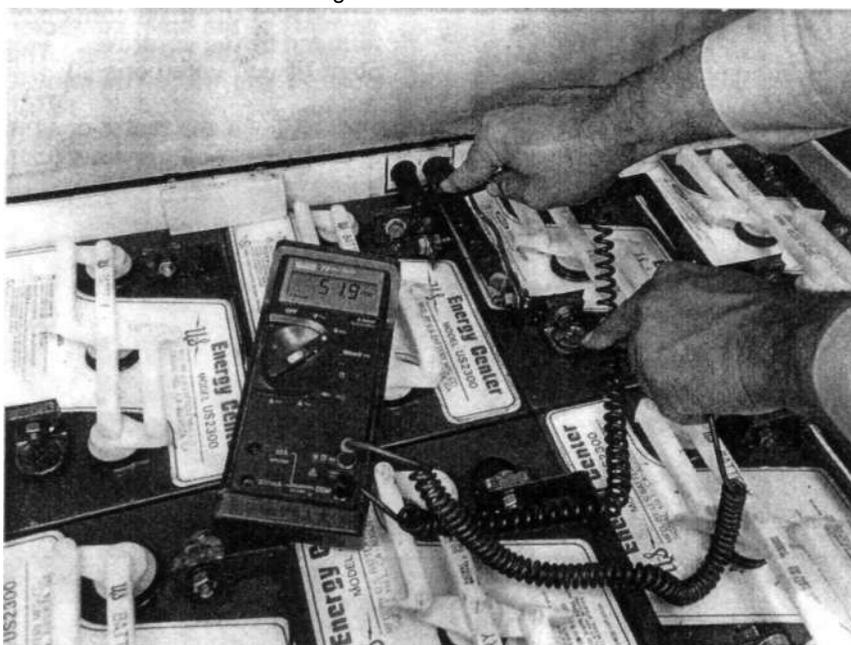
Checking battery pack voltage with a voltmeter.
