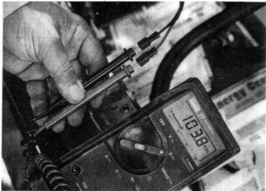
Checking for full pack voltage at a test point.
