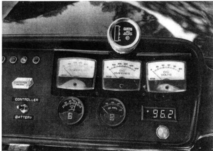
An LED bar gauge (top), panel meters (center), round automotive-style gauges (bottom left), and a digital gauge (bottom right). Note how the face on the leftmost panel meter is faded from the sun.
