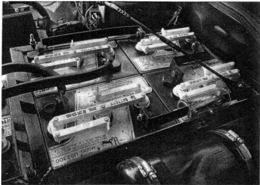
A battery pack using copper strap interconnects. Note fusible link in one interconnect.
