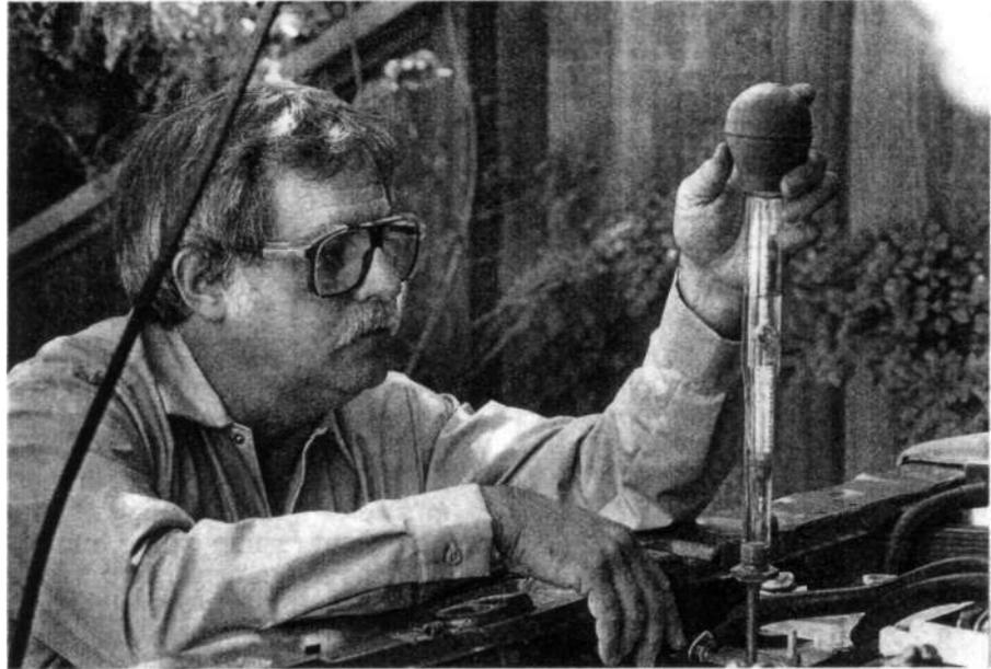
Testing specific gravity with a hydrometer.
