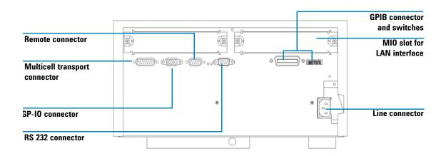
Figure 3 Rear view of spectrophotometer
