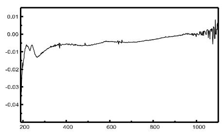
Figure 8 Spectrum taken with floating particles in the light path
