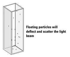
Figure 7 Floating particles in a cell
