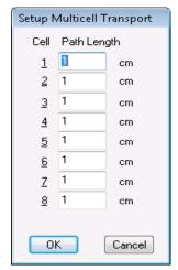
**3** To move your cell for the next measurement into the measurement position, click the cell on the Instrument Panel or choose Multicell Transport Position from the Spectrophotometer menu to access the Multicell transport Control dialog. In the Multicell Transport Control, press one of the position buttons to move the multicell transport.
