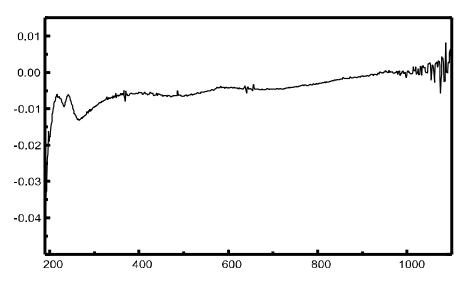
Figure 10 Example of a blank on water with bubbles causing a poor baseline
