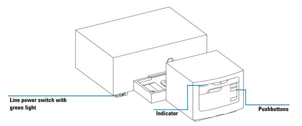
Figure 2 Front view of spectrophotometer
