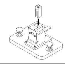
3 Lock the sample cell in place by pushing the locking lever back down.
