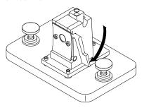
Utmost care should be taken when using small volume flow cells and particularly any cells with less than a 2 mm aperture. Here it is important that the cells are properly centered in the light path. The cell holder is designed for cells with 15 mm center height. If applicable, these cells should not be removed between the respective reference (blank) measurement and the sample measurement.
