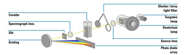
Figure 1 Optical system of spectrophotometer
