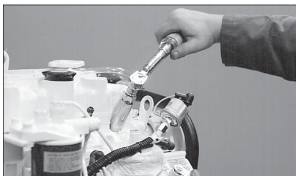
Figure 19: Reinstall injector. Torque to proper tightness.
