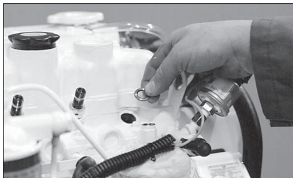
Figure 18: Remove and replace copper sealing washer.
