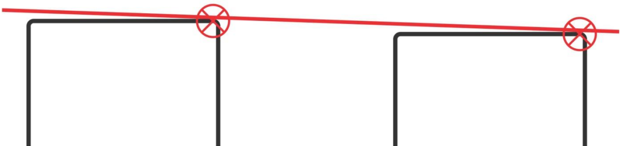
Figure 10: Tubular Inserts Flatness Inspection
