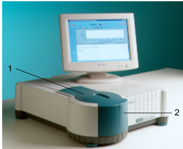
Figure 2-1 Cary 50 showing the sample compartment lid (1) and front panel (2)
