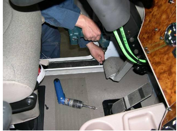
Figure 9 - Driver Door Scuff Plate Removal
