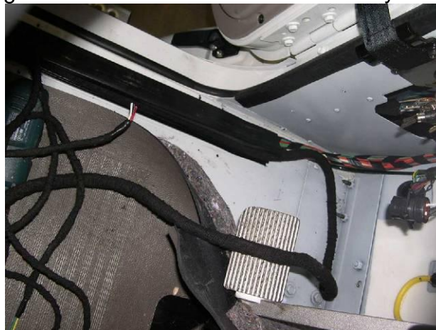
Figure 10 - Harness routed under Scuff Plate
