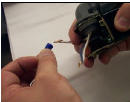
Removing the wire nuts
