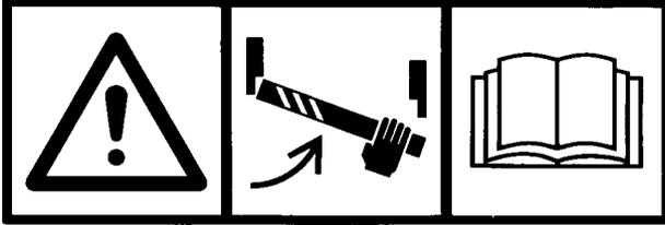
ISO Skip Support, when used, is pinned around the tipping ram rod to prevent the ram from closing.
