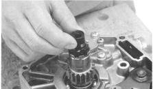
2 . Install the clutch bearing seat into the transmission mainshaft. (Set the bearing seat so its folded portion fits well with the crankcase so as to prevent it from rotating.)
