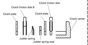
Degrease the oil completely not to remain oil on the clutch plates. Check that the clutch center and the clutch pressure plate fit in each other exactly.
