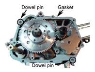
2 .Install the oil seal of the R crankcase cover COMP., and tighten the R. crankcase cover temporarily with the cap screw on the crankcase. Then tighten the cap screw in a crisscross pattern to the specified torque.
