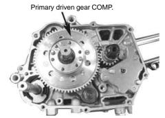
Place the vehicle on the flat surface with the maintenance stand properly. | 4 . Tighten the lock nut to the specified torque with the crankshaft being seated in detent.
