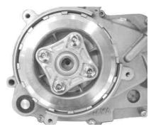
8 . Install the dry clutch cover referring to the instruction manual. Please adjust the clutch with the clutch lifter rod. Please put the engine oil.
