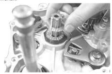
3 . Apply engine oil to the ball bearing of the primary driven gear COMP., and then the grease to the oil seal. And insert the primary driven gear COMP. into the mainshaft.
