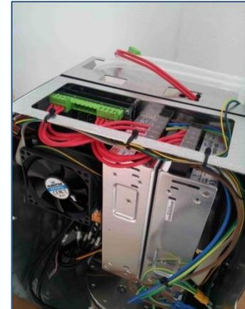
Cut the three fixing wires
