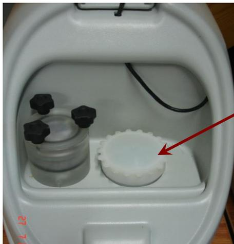
1- Open the front door and fill water tank with pure water (Deionized, ASTM II,  $<0,1\mu\text{S}</math>)$
