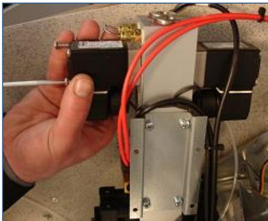
Unscrew the two screws at the top left and bottom right and remove the valve
