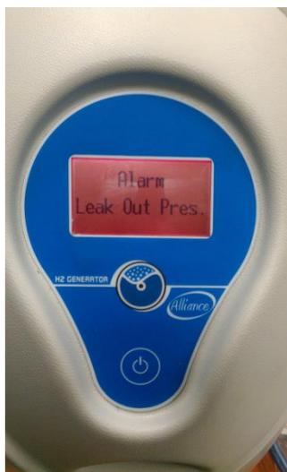
In case of serious anomalies, the display turns red, the buzzer is rapid and intermittent, a message identifying the problem is displayed and hydrogen production is immediately interrupted.
