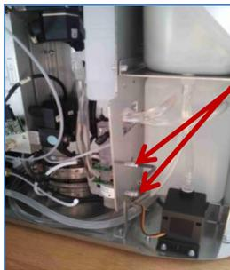
Unscrew the 2 screws with Allen key
