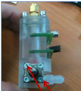
•Unscrew the two screws at the top left and bottom right and remove the valve
