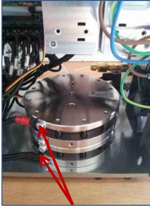
Unscrew the two screws on the cables of the cell power
