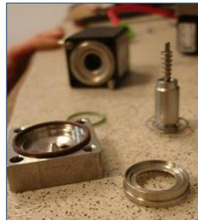
Then unscrew the remaining two screws and clean the internal components after verification of the presence of impurities
