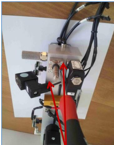
Unscrew the two screws at the top left and bottom right and remove the valve
