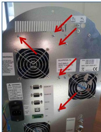
Unscrew the five screws on the rear panel
