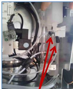
Disconnect pipes on quick connections
