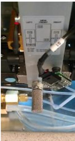
1- Remove the grey silencer and exchange it by a cap
