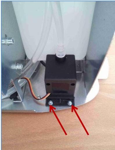
Unscrew the two screws located below the generator
