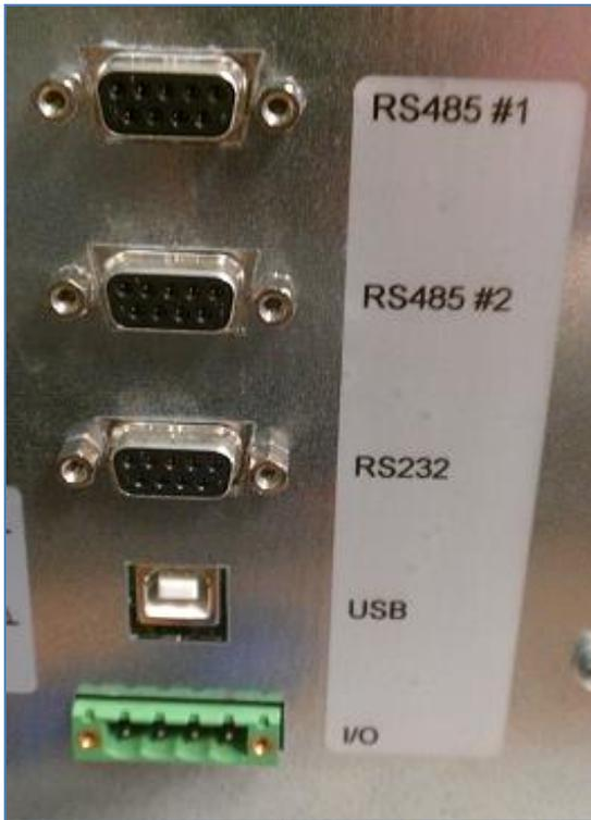
Connect the RS-485 controller with the BOX of 485 # 1 of the first generator and the RS 485 to RS # 2 of this 485 # 1 of the second and so on until the last generator.
