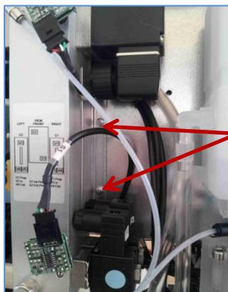
Unscrew the four mounting screws
