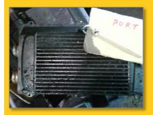
This charge air cooler core, removed from a high-speed engine after approximately 4000hrs operation, is heavily fouled on the air side with oil residue from the closed crankcase ventilation system. Its heat transfer capability is reduced by approximately 60% resulting in higher engine fuel consumption, elevated exhaust temperatures and impaired performance. Removal and cleaning each 1000hrs of operation is now part of the owner's maintenance schedule.
