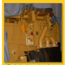
The duplex charge air cooler on this new 4500bKW marine propulsion engine is designed to remove 2000kw of heat from the combustion air before enters the cylinders. Note the separate connections for the low temperature and high temperature core sections. A pressure differential switch is fitted to provide a signal to the ship alarm system that cleaning is required.
