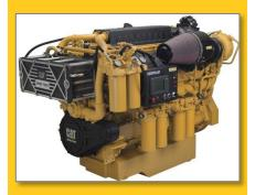
The charge air cooler core on this high-speed marine diesel is located under the black cast metal housing on the top of engine. The core is accessible by removing the top of the housing and disconnecting the air and cooling connections. The closedcrankcase ventilation system requires that the core is monitored intensively for efficiency and cleaned regularly to preserve engine performance and emissions compliance.
