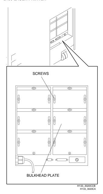
**[6]** Use a T15 TORX BIT to remove the SCREWS and all BULKHEAD PLATES.
