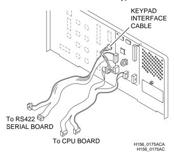
The following table shows the connector pinnout list for the KEYPAD INTEFACE CABLE. This CABLE is for the MIM 100 with the bulkhead with the RELAY BOARD. See the KEYPAD INTEFACE CABLE in the graphic below.
