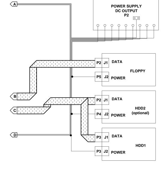
Video Interface of the MIM 100 with new CPU Board: Internal Cabling
