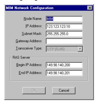
The Service Application allows you to view and modify the parameters for the TCP/IP and *Ethernet* BOARD that are necessary to configure the MIM as a device on the network. Although the RJ45 *Ethernet* connection is on the CPU BOARD of the MIM 50 and DP SERVER, you will use the LAPTOP to configure it.
