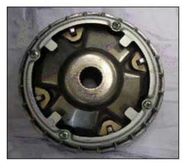
8. Clean the fixed drive pulley using compressed air.
