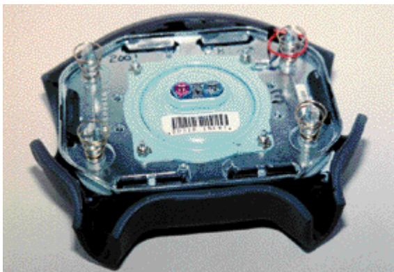
Dual stage airbag is identified by having two electrical connections.
