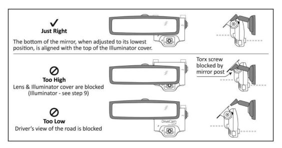
**Mounting Options:** Refer to the **DriveCam Mounting Guidelines (DRC 340)** if you're installing in a vehicle without a standard rear view mirror. The document provides additional details and diagrams about VER mounting in various vehicle types, including instructions for using the **Extended (Bulkhead) Bracket and RAM-Mount (Articulating) Bracket**. Government restrictions regarding the mounting of objects on the vehicle windshield and U.S. DOT exemptions are also covered.
