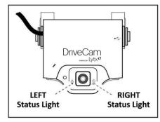
**Errors:** If the status lights **did not light at all**, check the wiring and fuses. If you see any other status light behaviors, contact Lytx Technical Support at (866) 910-0403.
