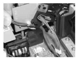
**17.** Remove three (3) screws from the fuser chassis.
