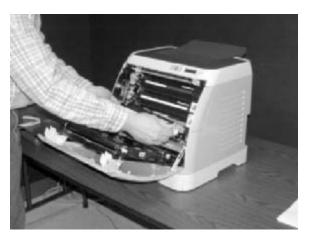
**3.** Remove the new print cartridge from the bag. Place the used print cartridge in the bag for recycling.
