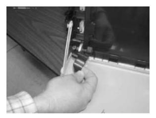
**10.** Remove one (1) grounding screw from the ETB harness.
