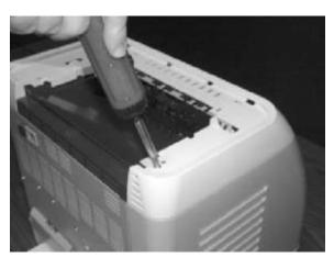
7. Remove one (1) screw from the inside upper cover (RC1–5178–000CN) and then remove the black output guide.
