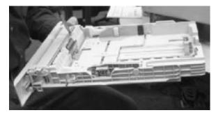
2. Remove two (2) screws that attach the separation pad.
