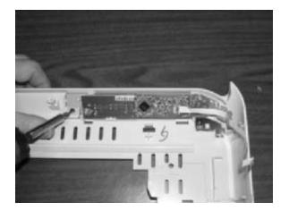
9. Remove the control panel assembly (RM1–1983–000CN).
