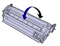
**5.** Remove the orange shipping locks and the orange shipping tape from the new print cartridge. Discard the shipping tape and shipping locks according to local regulations.
