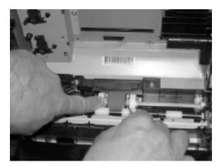
6. Rotating it towards the back, remove the paper pickup roller (RC1-5440-000CN).
