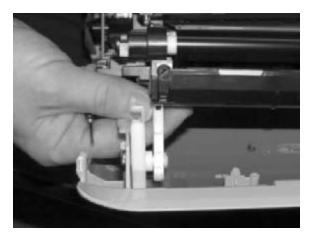
7. Remove the screw on the right white plastic catch, and then remove the plastic catch.
