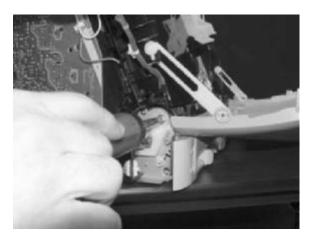
**14.** Using needle-nose pliers, remove the hinge left cam (RC1–4249–000CN) and the right hinge cam (RC1–5311–000CN).
