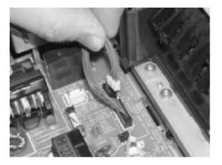
**16.** Remove the wiring harness.
