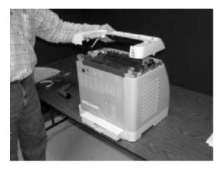
**10.** Remove the output tray by releasing the tabs.
