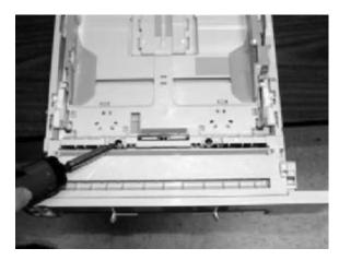
3. Remove the separation pad assembly (RC1–5356–000CN).
