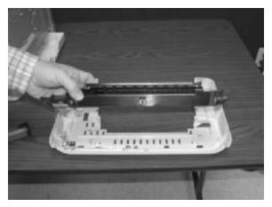
8. Remove two (2) screws from the control panel.
