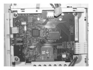
6. Lifting it up, remove the formatter.
