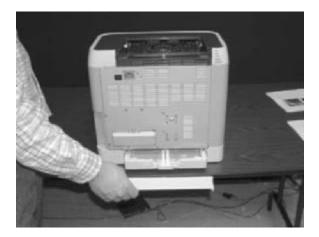
2. Remove nine (9) screws from the rear plate (RC1–5227–000CN).
