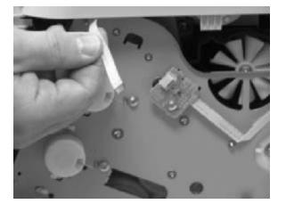
5. Lift up and remove the upper face cover (RC1-5173-000CN).
