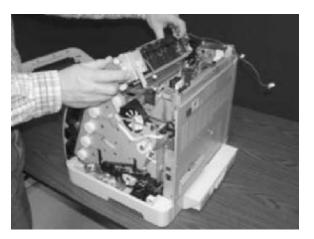
Use the following procedure to replace the fuser.
