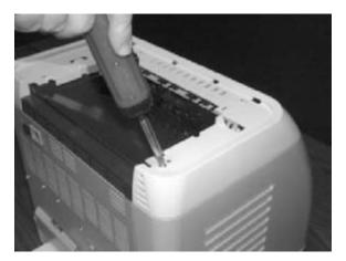
9. Lift up and remove the face-down cover (RC1–5173–000CN).
