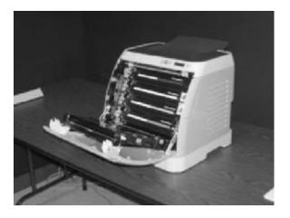
CAUTION Do not place anything on the transfer belt (ETB), which is located on the inside of the front door.
