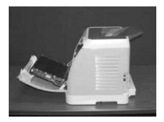
**4.** Remove the right cover (RM1–1858–000CN), carefully twisting the front edges of the side covers outward to remove.
