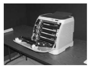
2. Remove the print cartridges.
