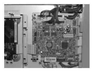
Remove four (4) screws from the DC controller. 5.
