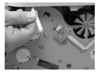
6. Insert a screwdriver to loosen the release tab on each side of the upper face cover.
