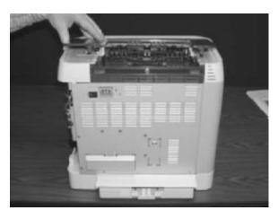
8. Remove four (4) screws from the upper cover (RC1–5176–000CN).
