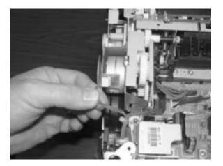
**12.** Open two (2) clips and remove one (1) clip to remove the fuser connector.
