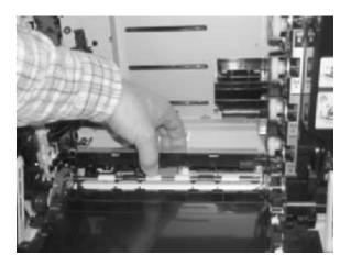
5. Use a small screwdriver to pull back on the tabs.
