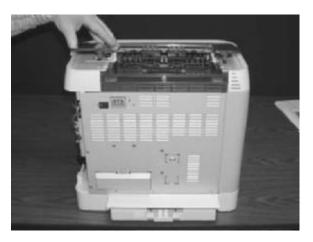
6. Remove four (4) screws from the upper cover (RC1–5176–000CN).
