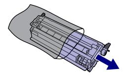
4. Grasp both sides of the print cartridge by the blue handles and distribute the toner by gently rocking the print cartridge from back to front.
