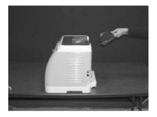
**3.** Remove the right cover assembly (RM1–1858–000CN), carefully twisting the front edges of the side covers outward to remove.
