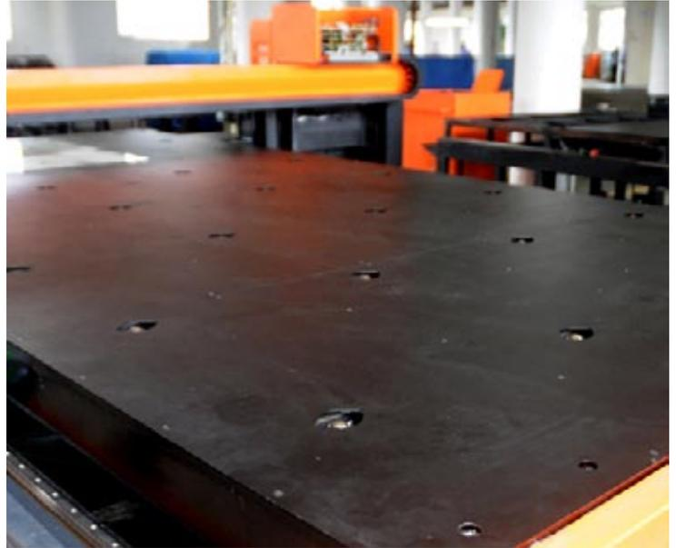
Here you can see there are two kinds of tables, the one that works with vacuum, at the right, and the one that is especially designed to print on glass, at the left.
