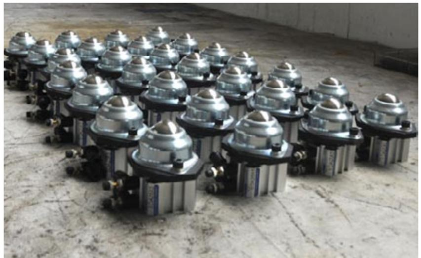
**SkyJet glass lifter balls that allow you to raise and lower the glass sheets easily.**
