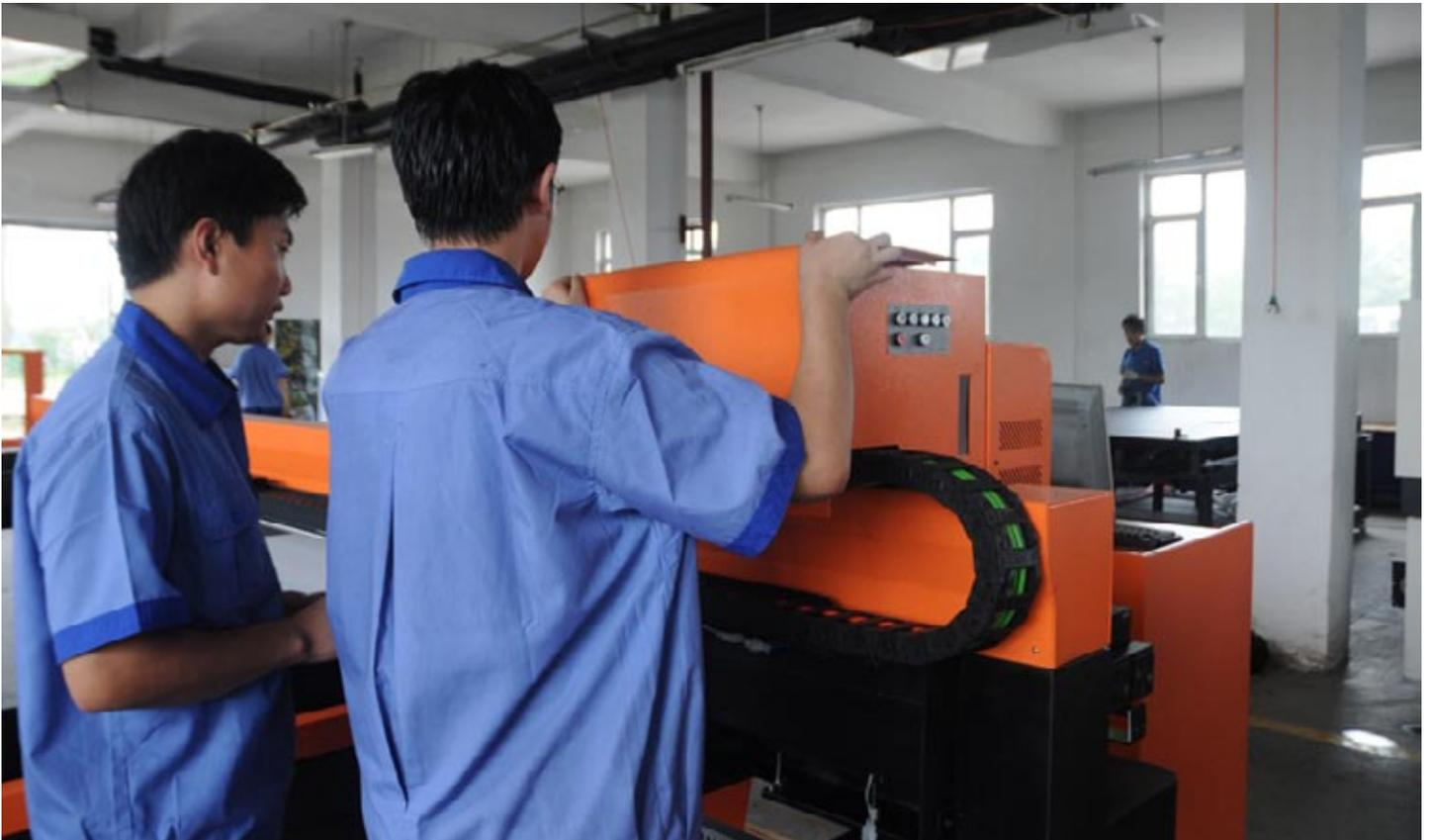
*In the FlatMaster what moves is the gantry, and if the object you are printing is not as wide as the full width of the printer, the printhead carriage can hover only over the length of your media.*
