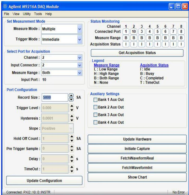
**Figure 9** Setting the M9216A for Multiple Channel acquisition
