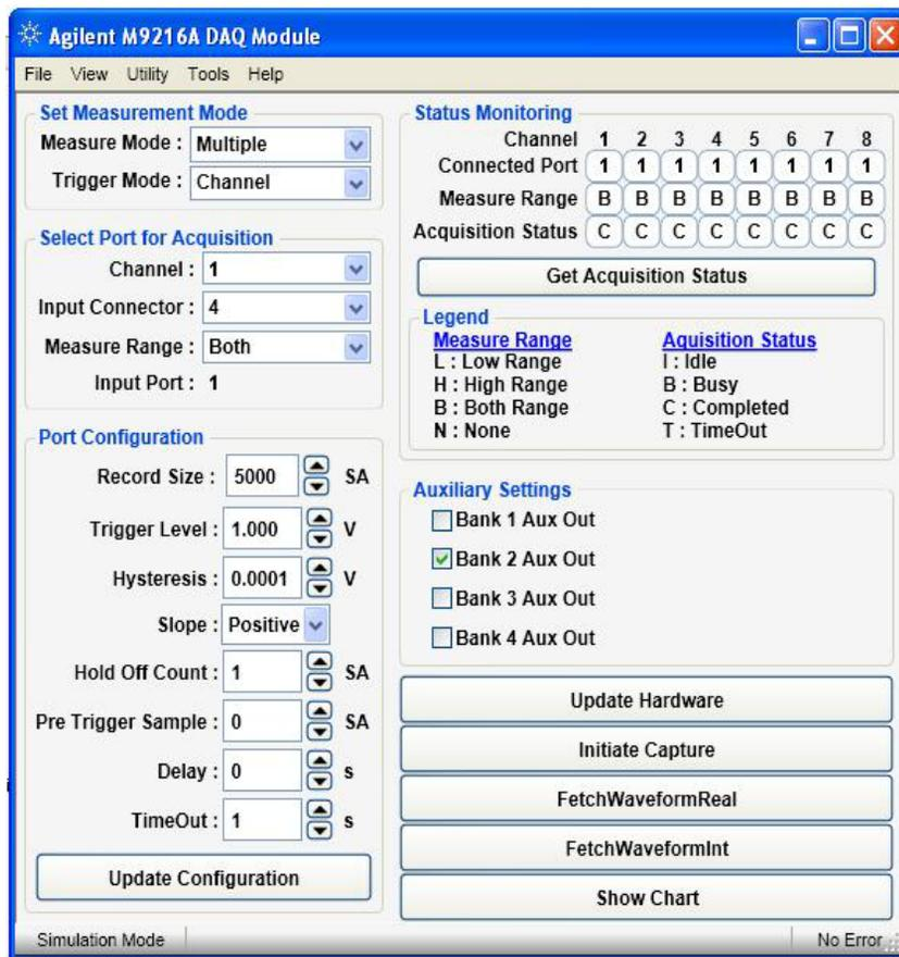
**Figure 12** Setting the auxiliary output ports
