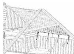
**16e** Follow steps 16b-16d and install a Roof Panel and Roof Support on opposite side.
