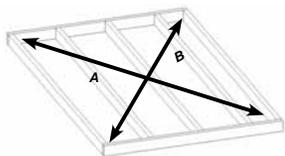
**Square up the frame by measuring from corner to corner. Measurement A should equal Measurement B.**
