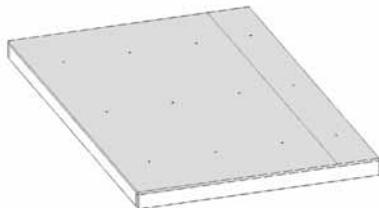
**Drill 3 evenly spaced 1/2" drain holes in plywood between each 2" x 4" joist.**
