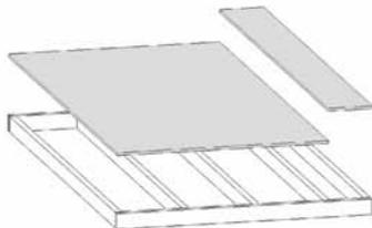
**Cut last sheet of plywood to fit remaining space (10" x 93.5") on frame. Nail plywood in place.**
