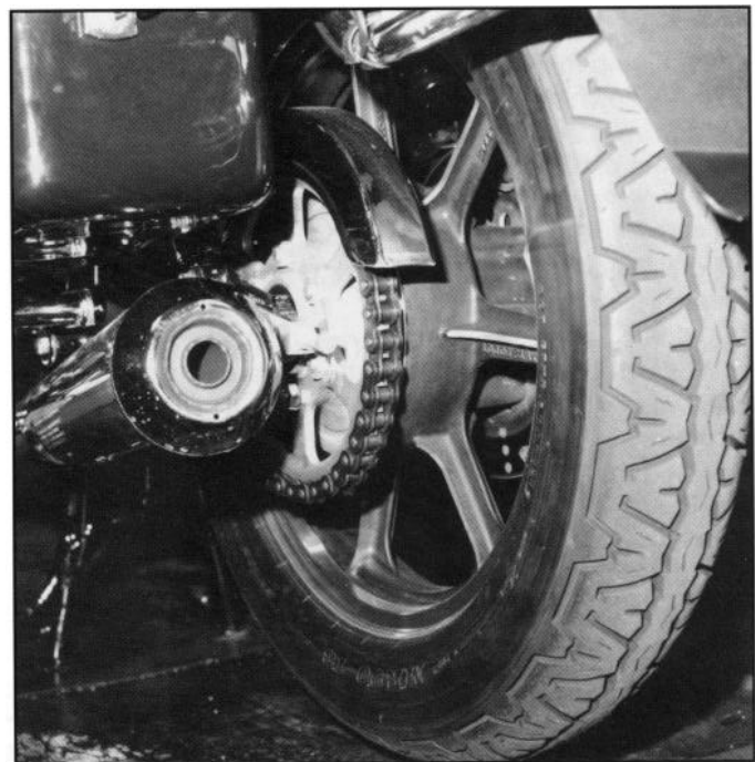
Proper chain tension and wheel alignment are key.
