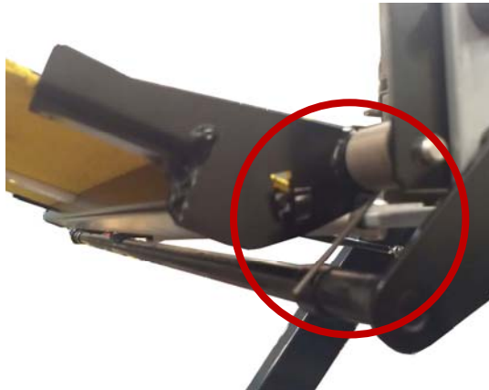
FIGURE 2-10. UNHOOK BRIDGEPLATE SPRING
