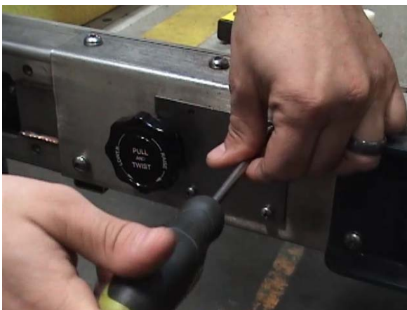
FIGURE 4-9: REMOVE MANUAL RELEASE COVER PLATE AND RH ROLLSTOP COVER
