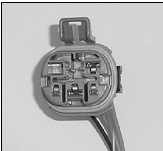
FIGURE 7.5 Fuel Pump Relay Connector
