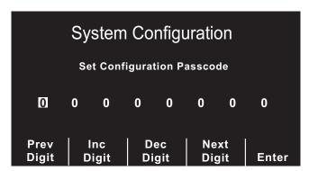
Pressing the **Prev Digit** softkey moves the highlight left to the previous entered digit. Pressing the **Inc Digit** or **Dec Digit** softkeys increments or decrements the selected digit. Pressing the **Next Digit** softkey moves the highlight right to the next digit to be entered. Pressing the **Enter** softkey selects the values that have been entered and returns to main configuration menu.
