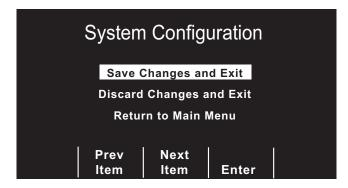
Press the **Prev Item** or **Next Item** softkey to scroll the highlight to the desired function. Press the **Enter** softkey to activate the selected function.
