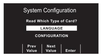
To move the highlighted area from LANGUAGE to CONFIGURATION and vice versa, press the **Prev Item** and **Next Item** softkeys. Press the **Enter** softkey to begin reading and storing the language settings or configuration settings from the user installed memory card.
