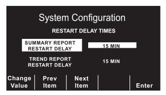
Pressing the Change Value softkey will scroll the highlight through the available delay times.
