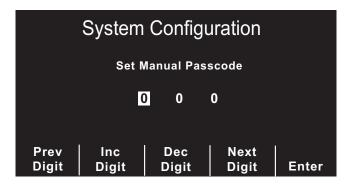
Pressing the **Prev Digit** softkey moves the highlight left to the previous entered digit. Pressing the **Inc Digit** or **Dec Digit** softkeys increments or decrements the selected digit. Pressing the **Next Digit** softkey moves the highlight right to the next digit to be entered. Pressing the **Enter** softkey selects the values that have been entered and returns to main configuration menu.
