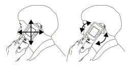
If your HA has a telecoil, activate its switch, then also rotate the handset as illustrated to align the telecoils. **Note:** Some automatically switched hearing aids may need an auxiliary switching magnet.
