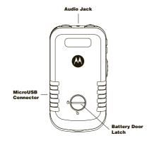
Your phone is designed to withstand being exposed to water for up to 30 minutes, and up to a depth of one meter. In order for your phone to be water resistant, the battery door must be properly attached and locked, and the audio jack and microUSB connector must be properly sealed.
