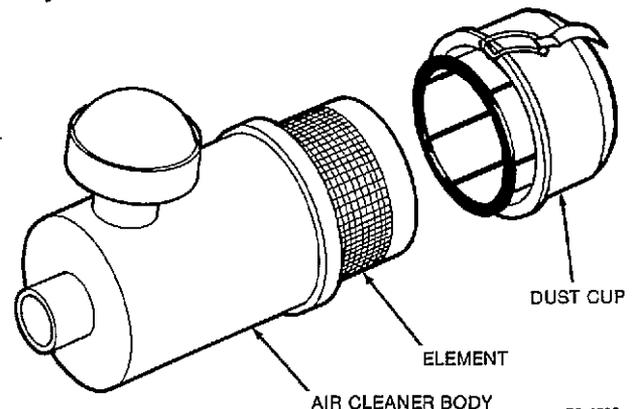
FIGURE 11. TYPICAL AIR CLEANER COMPONENTS
