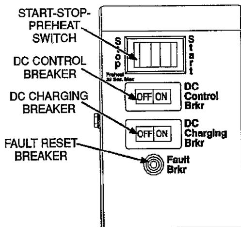
FIGURE 4. DC CONTROL BOX FRONT PANEL (REMOTE-MOUNT VERSION)
