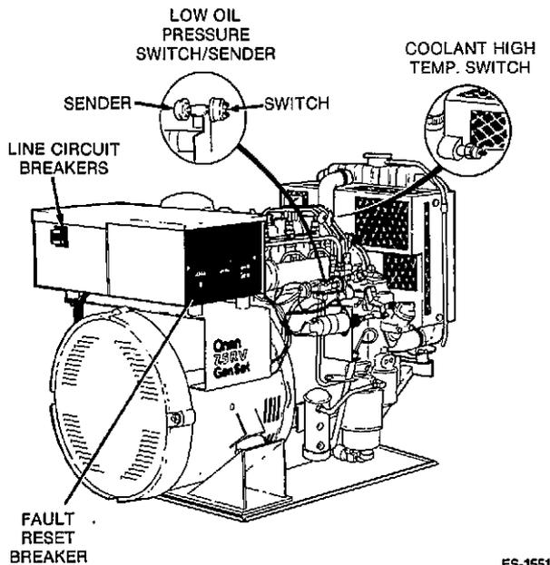
FIGURE 5. FAULT SENSOR LOCATION
