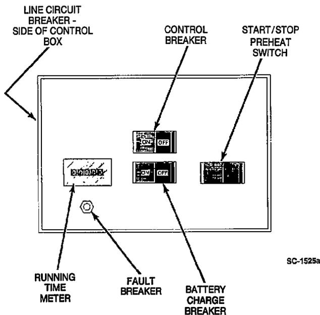
FIGURE 3. 7.5, 6.5 AND 6.0 DKD CONTROL BOX FRONT PANEL
