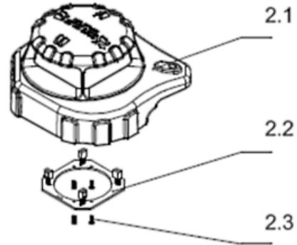
1. Remove Rechargeable #11 PCB (2-2) by removing retaining screws (2.3)
