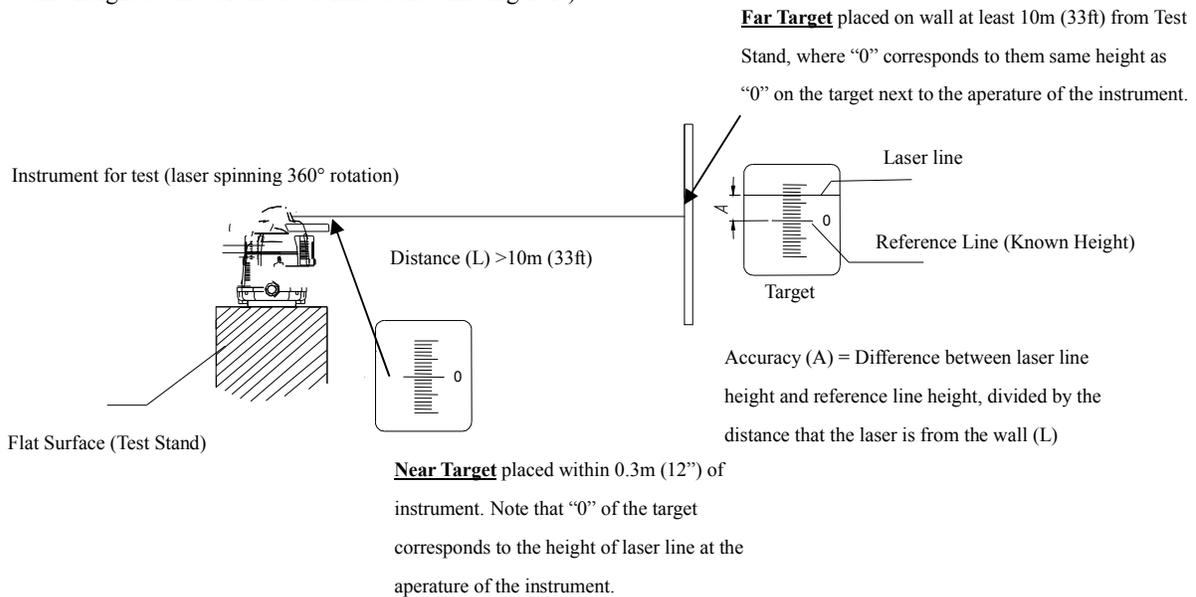
1. Place the instrument for test on the test stand (preconfigured from the illustration above) with handle facing the far target .
