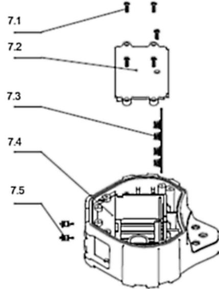
1. Disassemble Cover (7-2) by removing 5 retaining screws (7-1)
