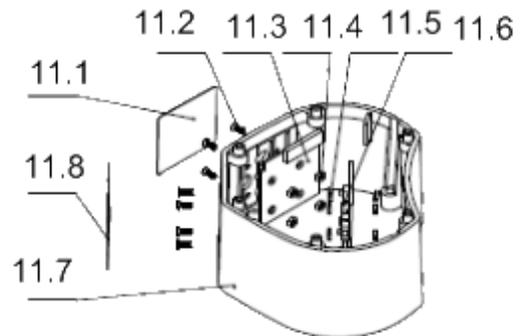
1. Remove keypads 1 and 2 (11-1) and (11-7) respectively, by peeling off of housing.
