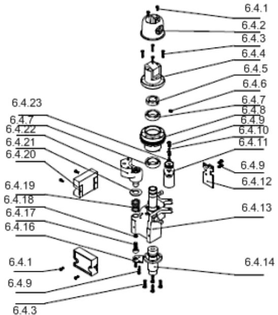
1. Disassemble Ball Gimbal Assembly (6-4-22) and Compression Spring (6-4-19) by removing retaining screw (6-4-17) and respective elastic gasket (6-4-18).
