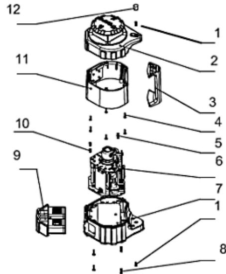
1. Remove Rechargeable Battery Pack (9) by turning retaining screw counter clockwise.
