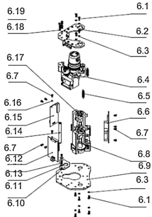
1. Remove #4 PCB (6-13) and #5 PCB (6-15) by loosening/removing retaining 6 screws (6-7) and 2 elastic gaskets (6-16) respectively.
