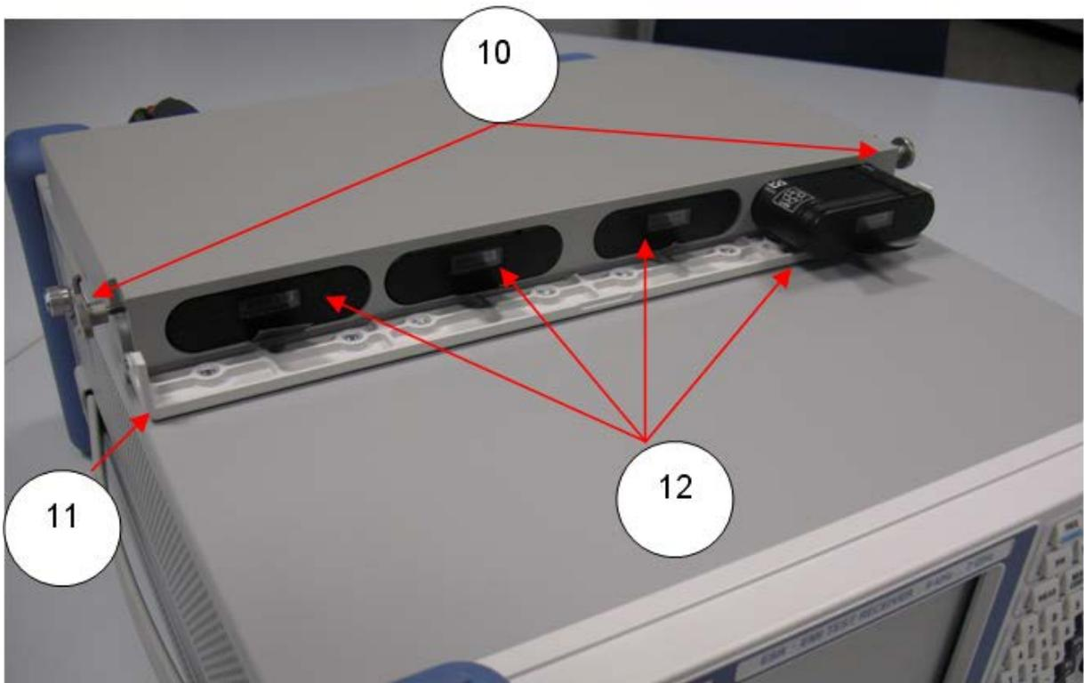
**Fig. 3-1: Battery compartment**
