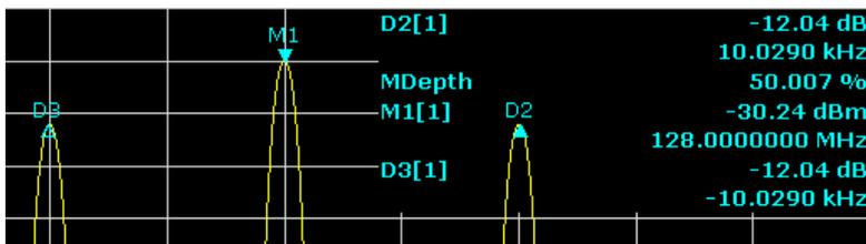
Fig. 6-7: Measurement of the AM modulation depth
