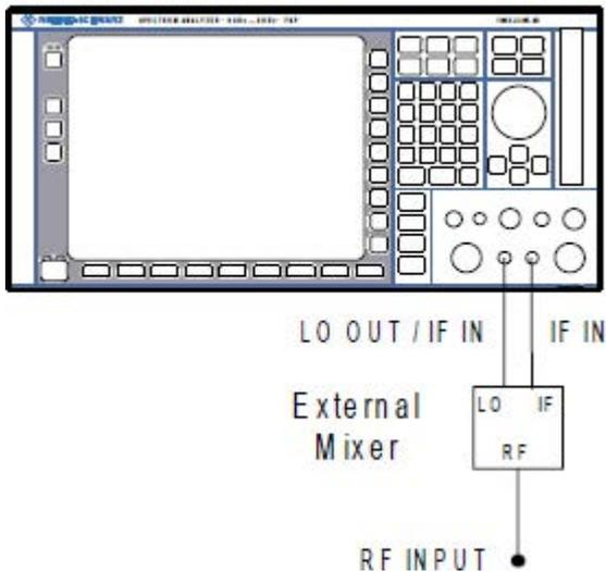
1. Connect the LO OUT / IF IN output of the R&S FSV to the LO port of the external mixer.
