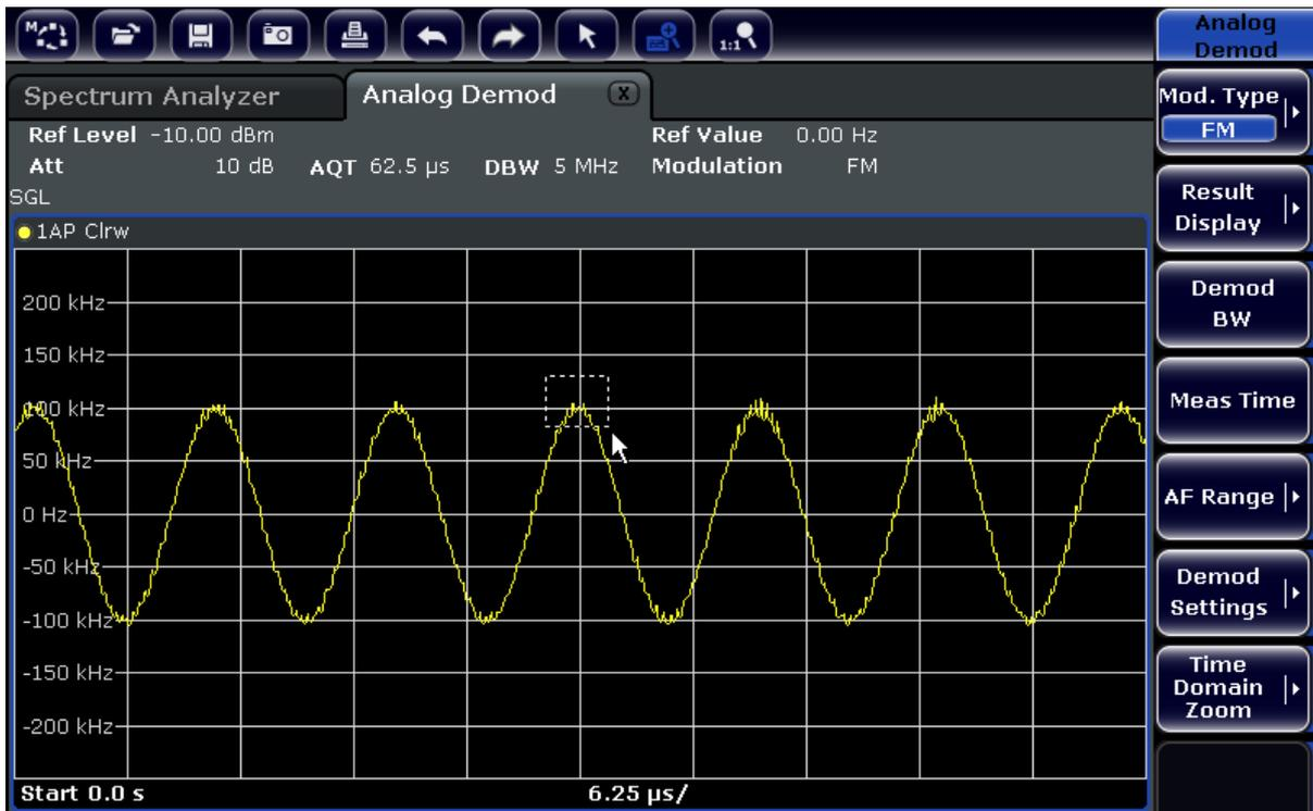
3. Drag the lower right corner of the rectangle (either via touchscreen or a mouse pointer) to define the area in the diagram to be enlarged.
