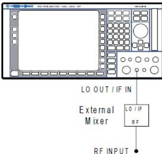
1. 1. Connect the LO OUT / IF IN output of the R&S FSV to the LO/IF port of the external mixer. The nominal LO level is 15.5 dBm.
