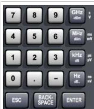
The keypad is used to enter alphanumeric parameters. It contains the following keys:
