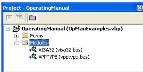
The modules `visa32.bas` and `vpptype.bas` can be found under `<VXIpnPath>\WinNT\include` (typically `C:\VXIpnPath\WinNt\include`). As an alternative, a reference to the `VISA32.DLL` can be added to the project.
