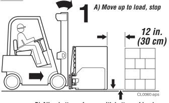
B) Align bottom of arms with bottom of load
