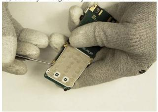
14) Separate LCD module from engine module.
