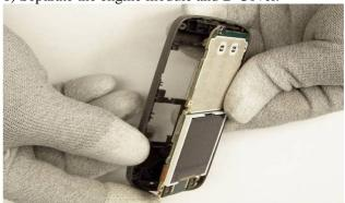
9) Lift and remove the antenna assy. Using the SS-93.
