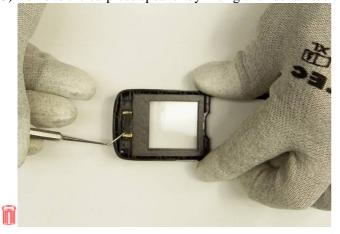
2) Using the SRT-6 start at the bottom of the phone and work around the edges to loosen the A-Cover.
