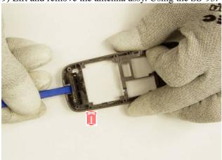
10) Lift and remove the IHF speaker using the SS-93.
