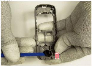
11) Push out and remove Mylar film.
