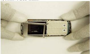
8) Separate the engine module and B-Cover.
