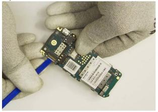
15) Carefully lift edge of key dome with dental tool.
