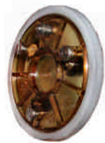
FIG. 6 Pumping piston removed completely
