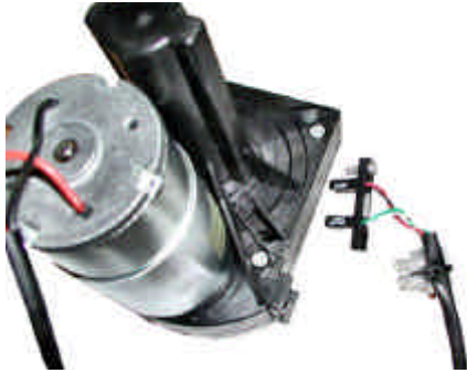
RATIOMOTOR: CONTROLLING BLOWING PISTON AND POSITION SENSOR
