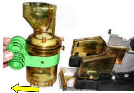
FIG. 2 Slide out the complete brewing chamber
