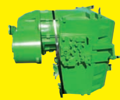
John Deere 8570 24-Speed Power Shift Transmission
