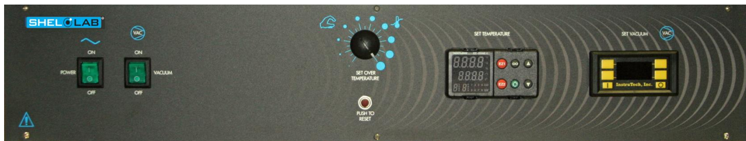
Figure 7: Control Panel SVAC9-2 and Watlow Temperature Controller
