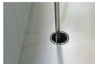
Figure 4: Cabinet Access Port – Back Deck of Oven
