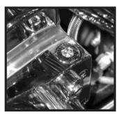
TRANSMISSION LUBRICANT The transmission lubricant level should be checked monthly. Big Dog Motorcycles recommends premium V-Twin motorcycle transmission lubricant. Synthetic lubricants are NOT recommended.
