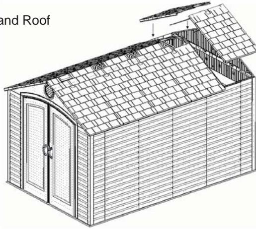
b. Add the last Center Roof Cap (117) and the End Roof Cap.
