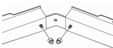
c. Slide a Threaded Rod through the Truss Support Brace and the top of the Truss Connector.
