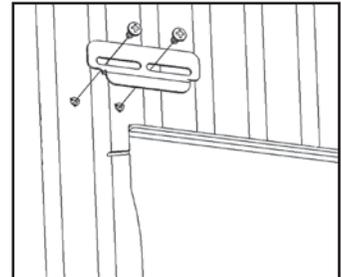
*Place Screw (TF) in this hole to keep window from sliding up too far. Insert until flush with the window*
