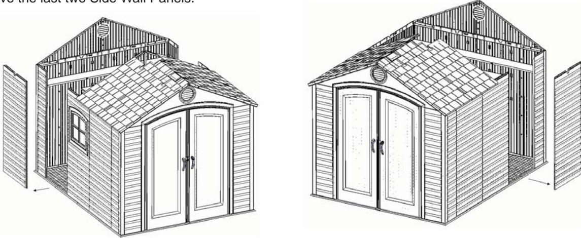
**Note:** If you're adding onto a side entry shed, remove the panels (in gray) from the side of the shed rather than removing the back of the shed. If you're adding on to both sides, remove the panels (in gray) from both sides of the shed (as illustrated), and follow the remaining steps.
