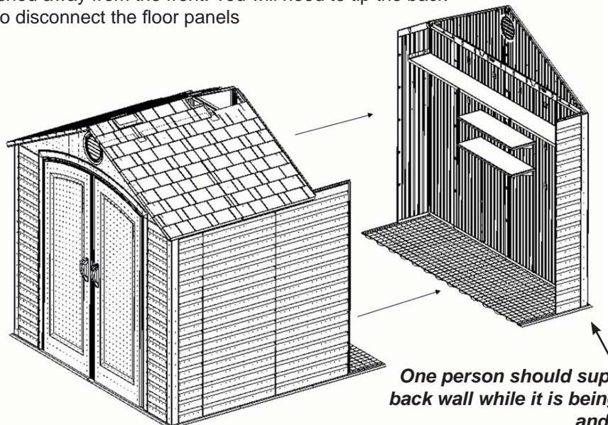
**One person should support the back wall while it is being tipped and moved.**
