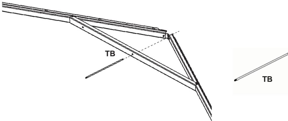
d. Secure the top and bottom of the Threaded Rod with a 1/4" Cap Nut (TD).
