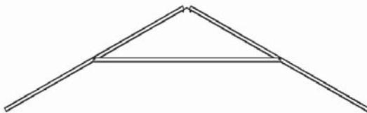
b. Use Truss Connector (TA) to attach Roof Truss Channels at top. Secure with Screws (TF) and Nuts (TE). Before completely tightening, lay assembly on its side to be sure Channels and Brace are parallel. Completely tighten all hardware.
