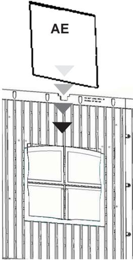
*Insert window with bent edge at top and pointing away from the wall.*
