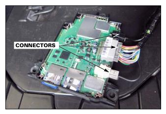
4. Connect the navigation unit to the PC with the USB cable as shown.
