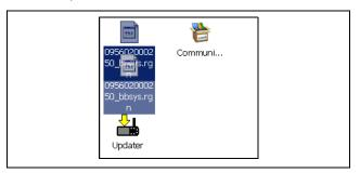
8. The *Updater* dialog box will open. Select *USB Device* and then click *OK* as shown. Keep holding the boot block button down during the navigation software update.
