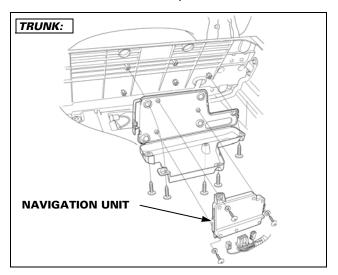
2. Remove the six screws and cover from the navigation unit.
