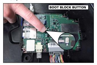
6. While holding the boot block button down, turn the ignition switch to the ACC position.
