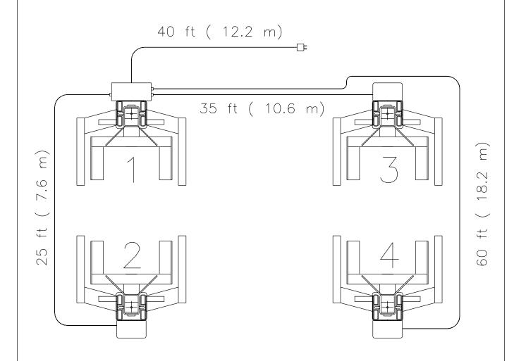
COLUMN CABLE CONNECTION SET OF 4 COLUMNS
