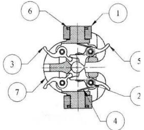
NOTE: The front of the Rear Latch (ref 3) must be on the inside of the back end portion of the Front Latch (ref 5). Once the Front Latch is installed, check to insure that both Front and Rear Latches open and close together when actuating Front Latches. If Rear Latches are pressed, both Front and Rear Latches open and close together. Then the opened Front Latches permit easy entry of rod into seat area of Rod Elevator. Do not use if not working properly.
