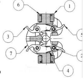
NOTE: The front of the Rear Latch (ref 3) must be on the inside of the back end portion of the Front Latch (ref 5). Once the Rear Latches are installed, check to insure that both Front and Rear Latches open and close together when actuating Front Latches. If Rear Latches are pressed, both Front and Rear Latches open and close together. Then the opened Front Latches permit easy entry of rod into seat area of Rod Elevator. Do not use if not working properly.
