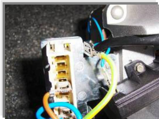
Plug the power cable. (220 V 50 Hz). After checking the motor operation, unplug the power cable soonest.
