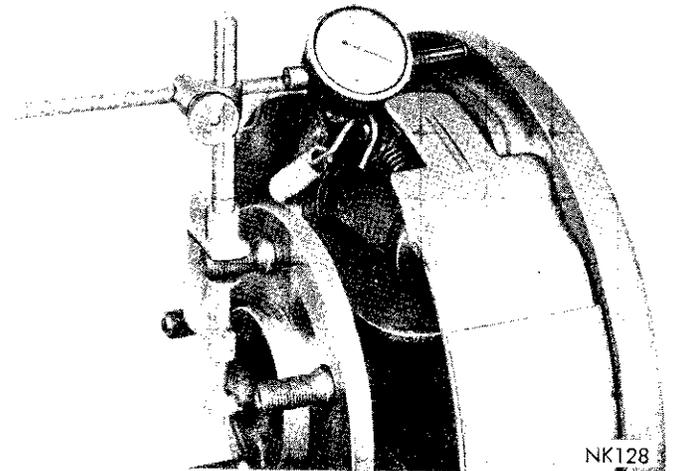
Fig. 15—Measuring Axle Shaft End Play
