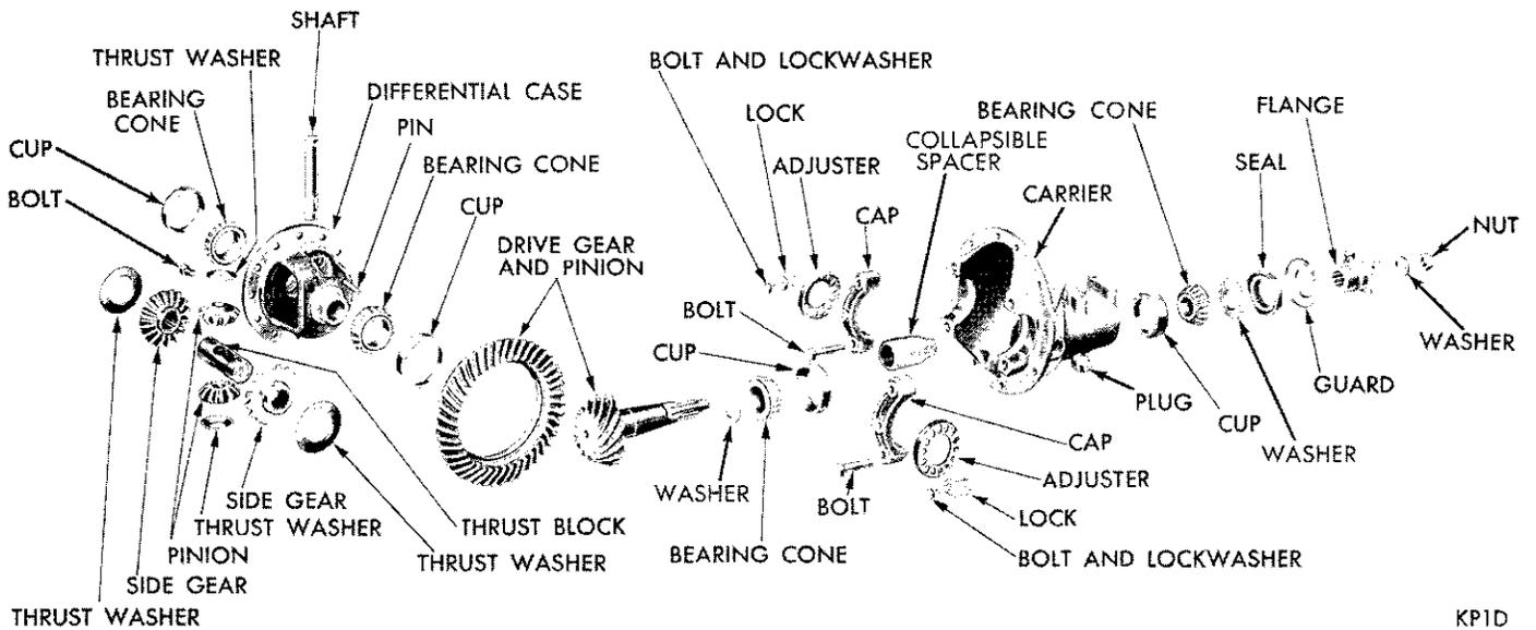
**Fig. 21—Differential Carrier Assembly (Large Stem Tapered Pinion)**
