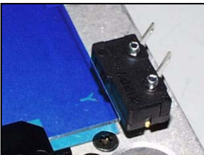
Fig. 76. Flag must engage microswitch
