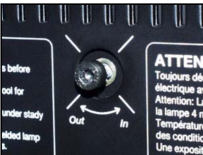
Fig. 45. Turn fully CCW
