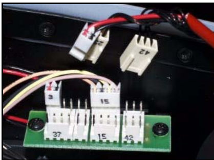
Fig. 2. Unplug right junction print
