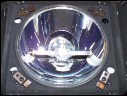
Fig. 44. Turn clips to free reflector
