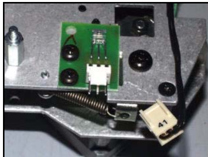
Fig. 62. Unplug light sensor
