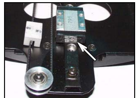
Fig. 17. Do not remove slide from rail
