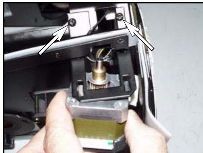
Fig. 15. Loosen bracket to remove motor
