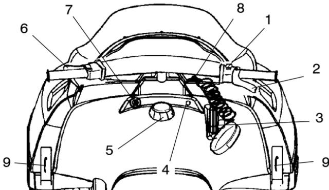
1. **Engine Stop Switch** - When the engine is running, you can push this button down and the engine will stop. The stop switch must be in the UP position to start the engine again.
