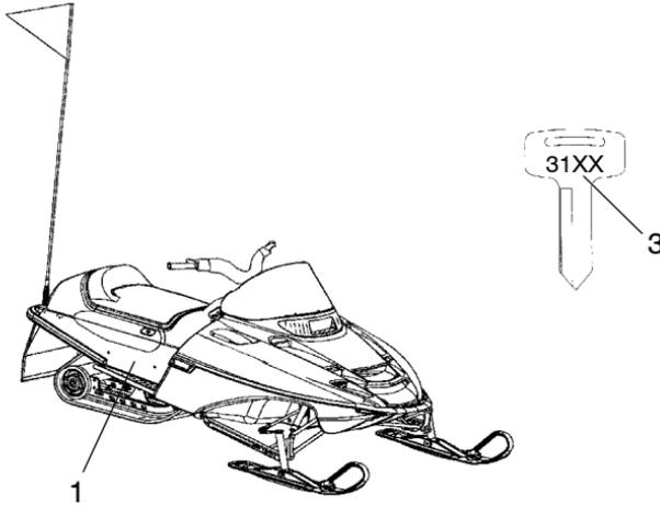
1. Tunnel VIN (lower right side of the tunnel)
