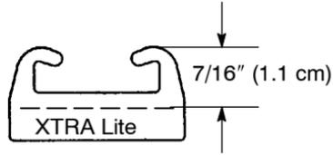
The slide rail is designed to operate in conditions with adequate snow cover to provide sufficient lubrication. Excessive wear may be due to improper alignment, improper track adjustment or machine operation on surfaces without snow. Take the machine to your dealer for slider replacement.
