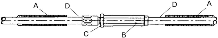
4. Check the actuator linkage to ensure there is adequate freedom of movement for positive brake operation and that all floating parts move freely and that all parts are mounted securely. Tighten hardware as required.
