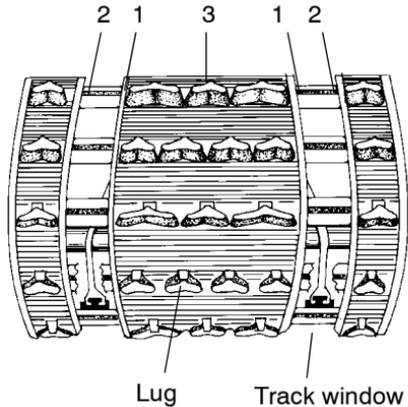
Check the track clips and tighten if loose. If any rod damage is found, the track should be replaced.
