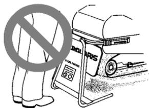
This snowmobile is propelled by a revolving track, which must be partially exposed for proper operation. Serious injuries may be caused by operator carelessness, resulting in hands, feet, hair or clothing becoming entangled in the track. Teach your child to respect this machine and all the moving parts. Stress that being properly seated keeps the child clear of the track.
