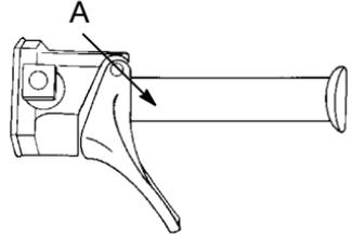
The throttle safety switch is designed to stop the engine whenever all pressure is removed from the throttle lever and the throttle cable or valve does not return to the normal closed position.
