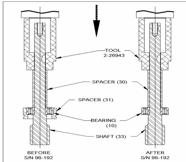
Figure 18. Pressing Spacer onto Bearing
