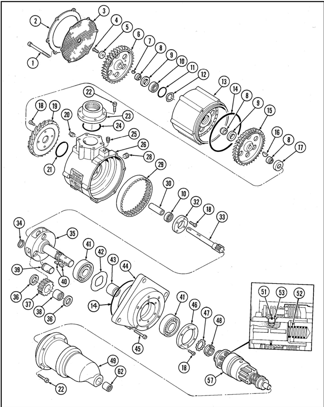
Figure 31. Illustrated Parts Breakdown (T112D/T121D, Standard Mesh)
