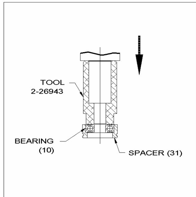
T100 is the original design (SN: 9501-239 to 9611-191), press the spacer (31) onto the outer race of the bearing (10) per *Figure 18* by supporting the bearing outer race, and then press the bearing/spacer (10, 31) onto the shaft.
