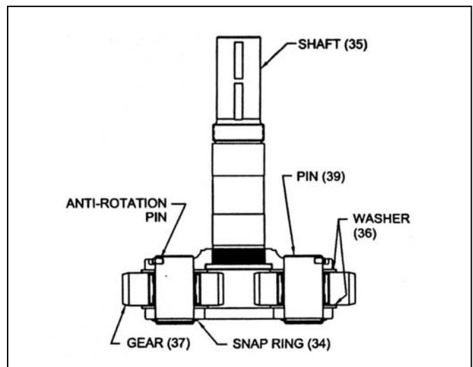
Figure 22. Planet Gear Carrier Shaft Assembly
