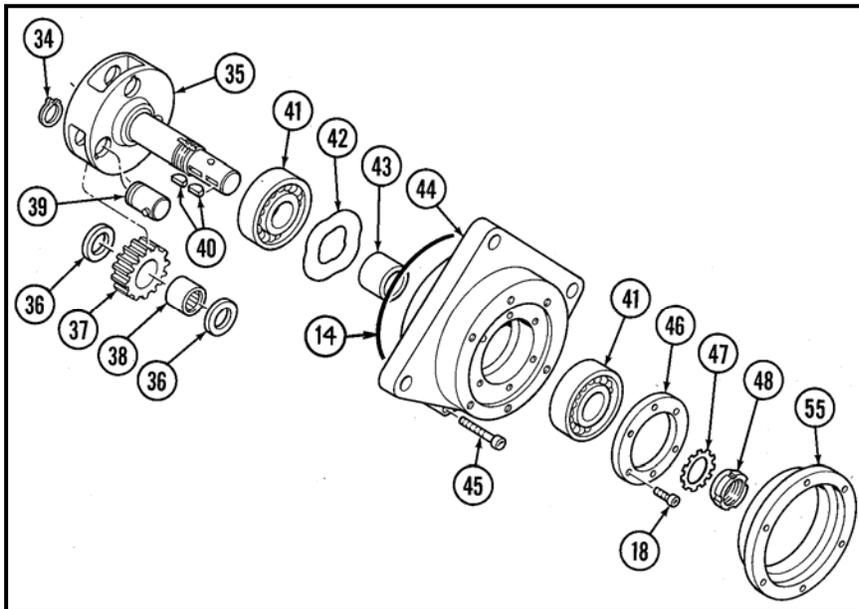
Figure 7. Gearbox Assembly (T112D/T121D LONG MESH)
