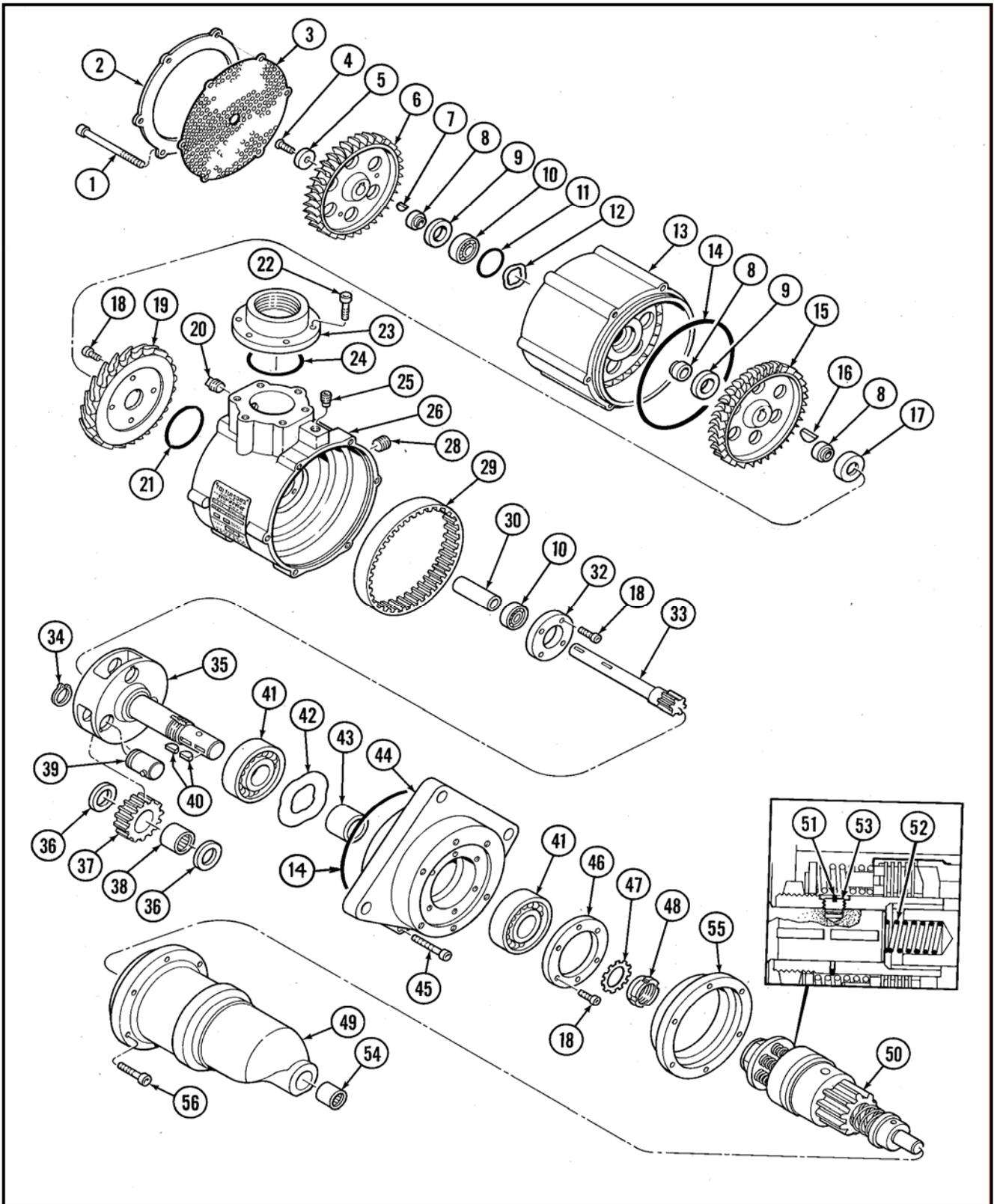
Figure 32. Illustrated Parts Breakdown (T112D/T121D, Long Mesh)
