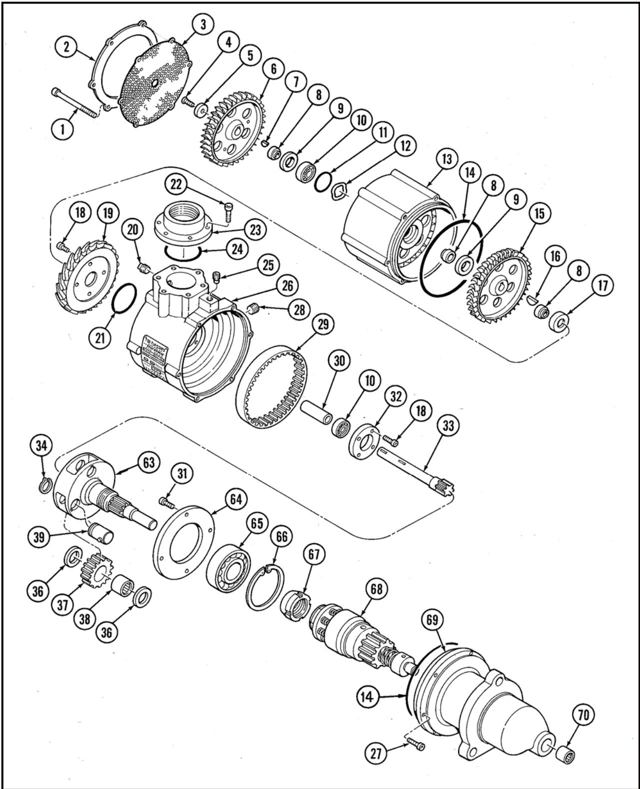
Figure 33. Illustrated Parts Breakdown (T106F/T112F)
