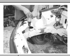
Slide the bracket back on the frame rail and thread the two bolts down through the bracket and out the bottom. Tighten the bolts to about 10ft/lbs of torque. Be careful to check the alignment of the bracket so the bolts thread easily all the way through the bracket. Do not over tighten.
