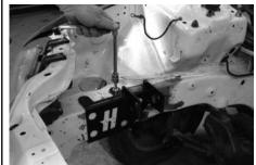
8 Using a wrench to keep the bolt from moving install the 10mm Nyloc nuts and tighten them to 36 ft/lbs of torque.
