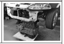
Once the engine is in the bay, but before the car is lowered completely, install the right-hand mount and bolt it to the transmission using the two 10mm x 50mm bolts and one 10mm x 30mm bolt. Leave all the bolts finger tight at this time. The 12mm x 100mm bolt, nut and washers will be used in Step 8.
