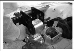
Lower the car the rest of the way to line up the left-hand mount. Install it by sliding the mount over the stud using the stock hardware to attach it. Next use the stock bolt to attach the mount to the frame rail bracket. Tighten all the left-hand mount hardware to 43 ft/lbs.
