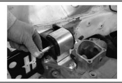
The Hasport rear bracket is designed to be used with either the EG/DC or EK chassis. For the EG and DC the hole indicated in the picture to the right will be used when attaching it to the rear mount.
