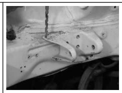
A chisel and hammer can now be used to finish removing the bracket. Once it is off use the die grinder with a sanding wheel to remove any left over material.
