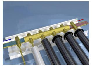
The condenser (large end of the heat-pipe) inserts though the heat-exchanger, but does not actually come into contact with the passing heat transfer fluid. The heat passes from the heat-pipe to the copper material of the exchanger and then into the passing fluid. This is an important point to understand should you need to change a tube and heat-pipe in the future. Tubes and heat-pipes can be changed without draining the system.
