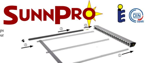
Once you have completed these steps you can position your collector frame and fix using an appropriate fixing method.
