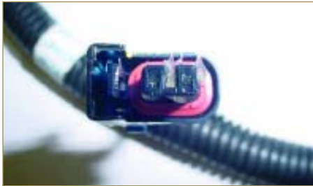
Properly applied lubricant
