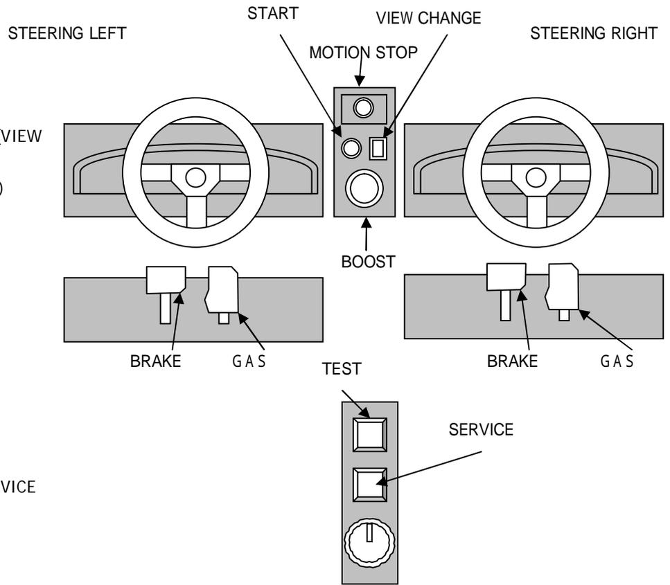
3. When all checks are completed, press the TEST Button and the SERVICE Button simultaneously. The GAME TEST MODE screen reappears.
