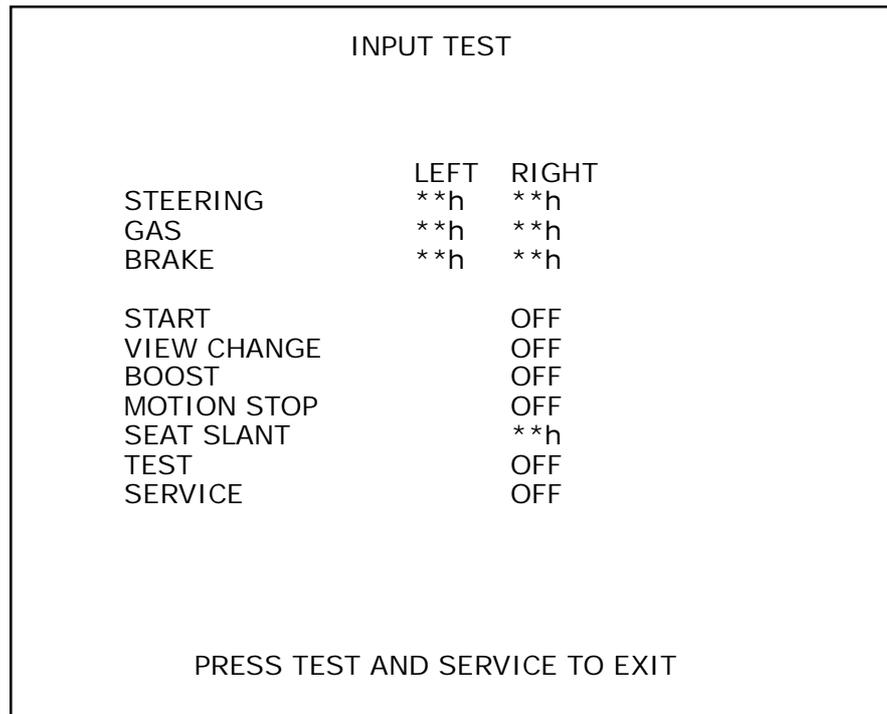
2. Manipulate each switch, etc., to check screen display.
