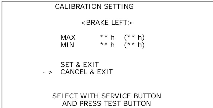
1. Press completely the brake pedal you are setting and then release it. The center number (hexadecimal) will change. MAX is the value when the pedal was pressed as hard as possible, and MIN is the value when the pedal was released. The number in parenthesis is the currently recorded setting value.
