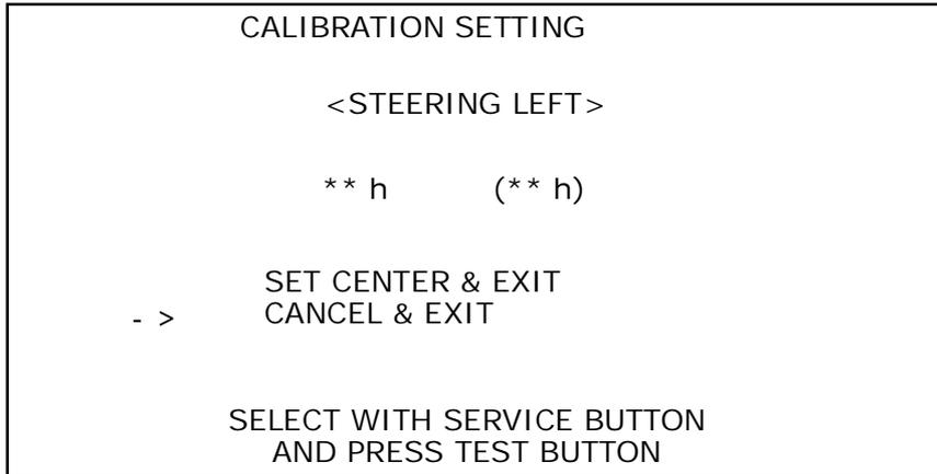
1. Hold the steering wheel to be set in the center position. The center number (hexadecimal) will change. The number in parenthesis is the currently recorded setting value. If it is significantly off the center position, the cursor will automatically select CANCEL & EXIT, and the setting will not be able to be made.
