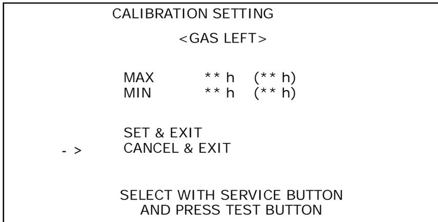
1. Press completely the gas pedal you are setting and then release it. The center number (hexadecimal) will change. MAX is the value when the pedal was pressed completely, and MIN is the value when the pedal was released. The number in parenthesis is the currently recorded setting value.
