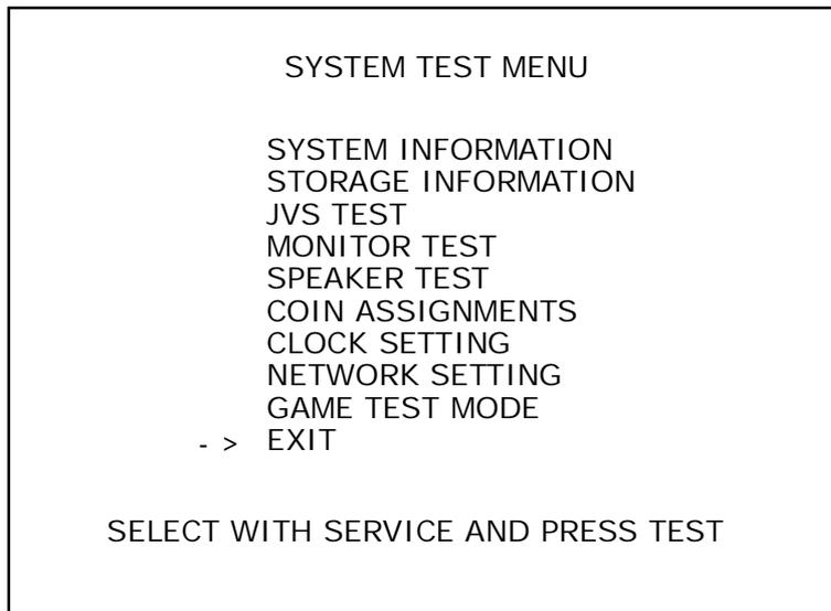
2. Use the SERVICE Button to move the cursor to the desired test item.
