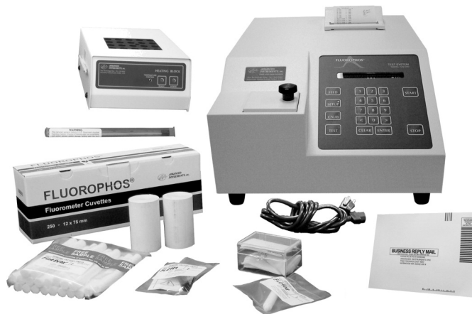
Figure 1-A: Model FLM200 Fluorophos® Test System and Supplies
