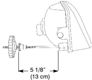
8. Carefully pull the assembly up and out of pod.
