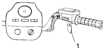
This ATV is equipped with Polaris Electronic Throttle Control (ETC), which is designed to reduce the risk of a frozen or stuck throttle. If the throttle cable should stick in an open position when the operator releases the throttle lever, the engine will stop, and power to the rear wheels will cease.
