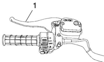
Always test brake lever travel and master cylinder fluid level before riding. When squeezed, the lever should feel firm. Any sponginess would indicate a possible fluid leak or low master cylinder fluid level, which must be corrected before riding. Contact your dealer for proper diagnosis and repairs.
