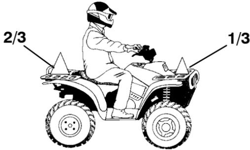
Your ATV has been designed to carry or tow a certain amount of load. Always read and understand the load distribution warnings listed on the warning labels, and never exceed the weights specified in your owner's manual supplement.
