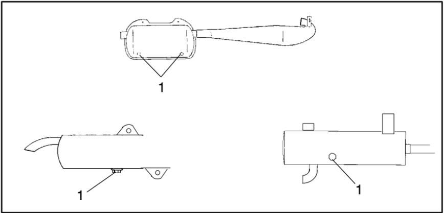
1. Remove the arrestor clean-out plug(s) (1) from the bottom of the muffler.
