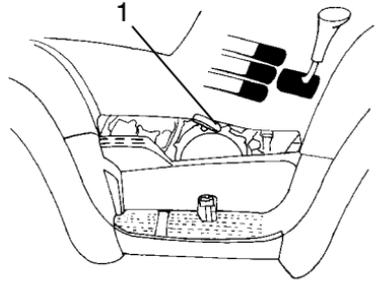
1. Position the vehicle on a level surface and engage the parking brake. See page 41.
