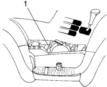
The transmission lubricant level should be checked monthly or 1000 miles (1600 km), whichever comes first. Transmission oil should be changed annually.
