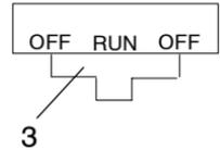
**Main Switch (2)** - To start the engine, slide the stop switch to the center “run” position and turn the main key switch clockwise past the “on” position. Release the key when the engine starts. **NOTE:** Turn off the main switch to end all electrical power to the vehicle, including the cooling fan and lights.
