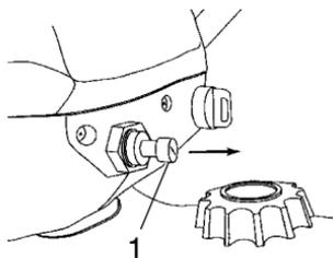
**NOTE:** The variable choke is fully on when the knob is pulled completely out. The choke is off
