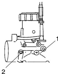
The following variations apply to air screw (2) adjustment for 2-cycle engines:
