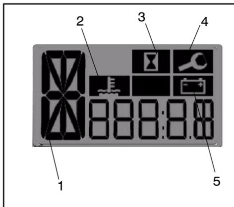
2. High Engine Coolant Temperature - Do not continue to operate the ATV if this warning appears or serious engine damage could result.
