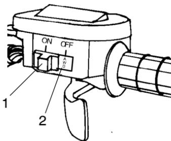
When in AWD, the front hubs will automatically engage any time the rear wheels lose traction. When the rear wheels regain traction, the front hubs will automatically disengage.
