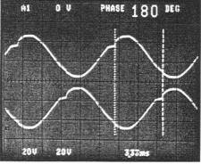
With the delta-time and voltage cursors, you can measure a waveform's parameters including phase.
