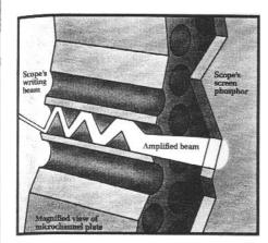
This MCP technology makes it possible to see a single sweep even at 500 picosec/div without a viewing hood. Even those difficult to find logic errors or metastability problems in a repetitive signal environment are easily seen.
