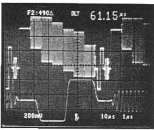
The 2467BHD automatically triggers on trilevel sync pulses used in high-definition video signals. Note: Line Count Readout Displays Field 2 – Line #490.
