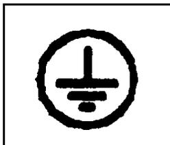
**Protective conductor Terminal** (IEC 417, No. 5019) This symbol designates the ground terminal for the mains protective ground. The wiring should be green/yellow in color.
